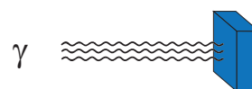
gamma: high energy photons, stopped by, dense material, such as concrete or water
